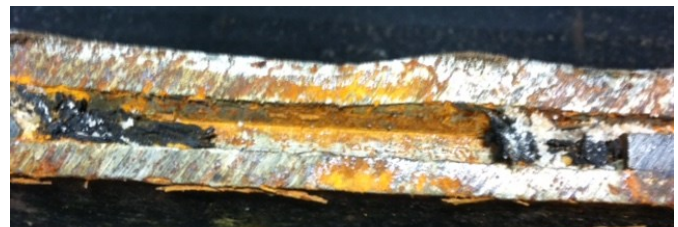
Standard Carbide - Fractured/Missing Carbide
